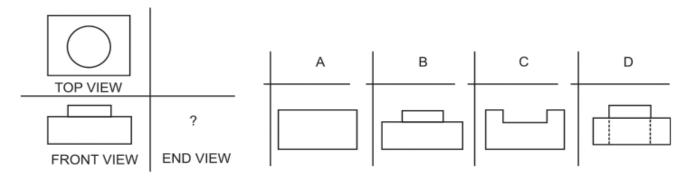
The front view shows that there is a smaller block on the base and that there is no hole.
