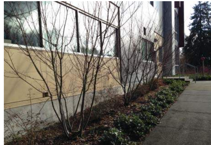
Avoid planting trees and plants too close to buildings, walkways, and entries. Appropriately placed plants will require less pruning, improve sight lines, increase safety, and reduce damage to structures and pavement.
